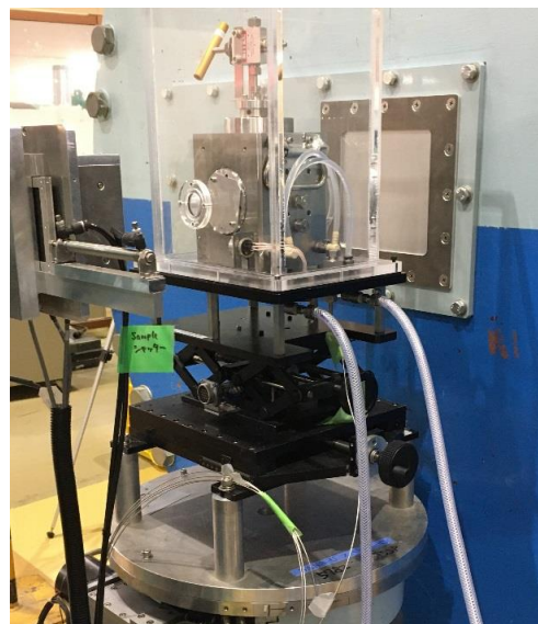
Fig. 1. A high-pressure cell installed at the SANS sample position for a test experiment.
